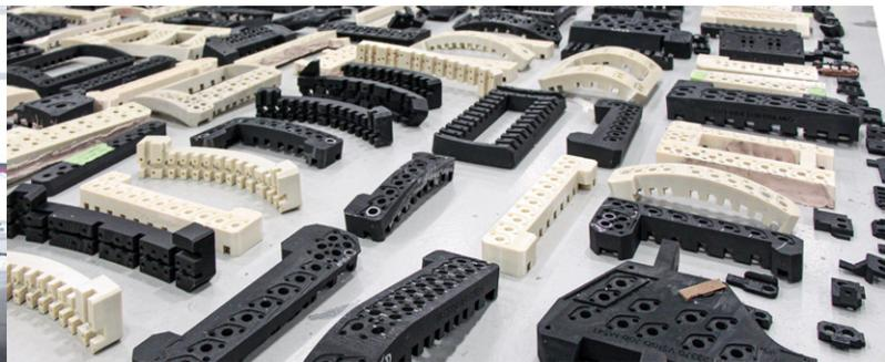
**Boom Supersonic used 3D printed flight control test rig tooling for its XB-1 supersonic jet. The printed tools resulted in a 90% cost and lead time savings over conventionally produced tooling.**
