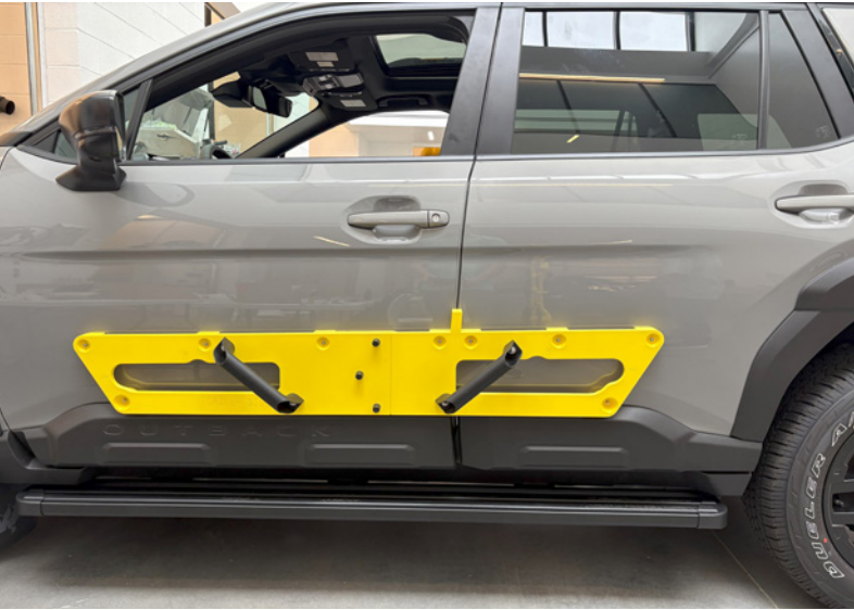
This view shows how the FDM tooling is used to correctly position the attachment of body side moldings.
