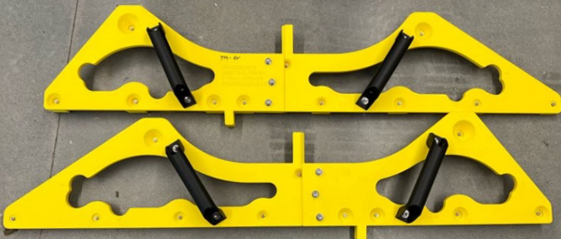
The positioning fixtures were printed with high-visibility yellow ASA material. The handles are standard off-the-shelf stock.
