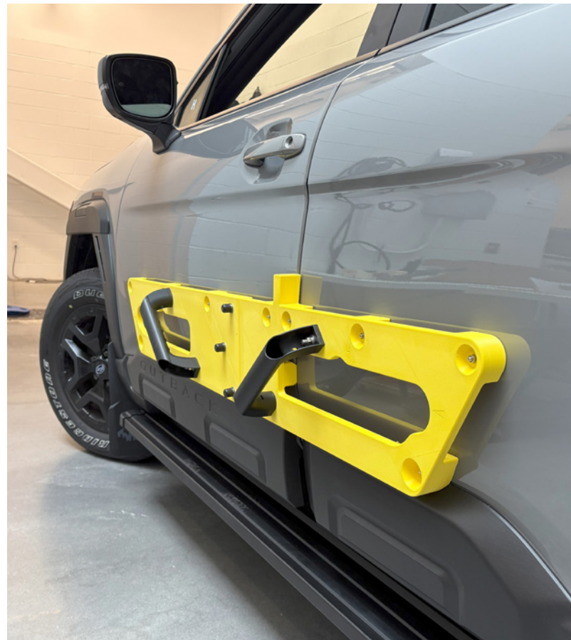
Magnets allow the tools to adhere to the car. Soft-touch pads bonded to the tools after printing prevent surface marring.
