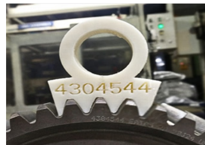
Two examples of gear teeth check fixtures printed on the F170 3D printer.
