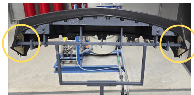
Two examples of 3D printed masks (highlighted) installed on a part in the paint fixture.
