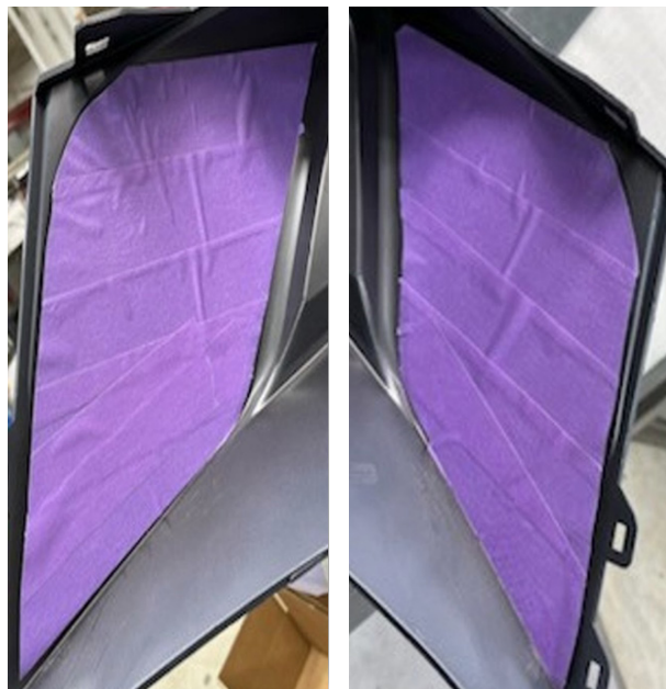
The tape applied to the 3D printed paint masks checks for masking effectiveness.
