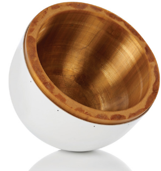
Figure 6-8: View of the composite part (white) on the FDM lay-up mold (amber).
