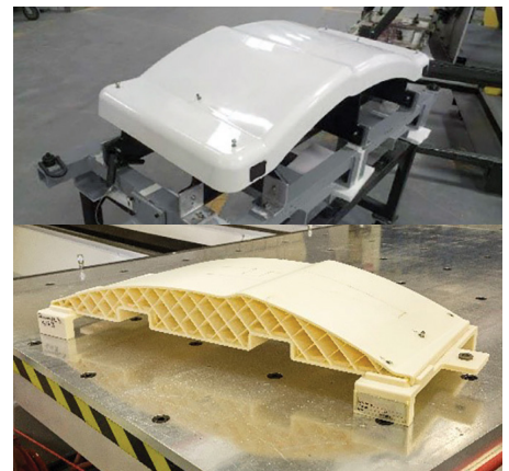
Figure 6-2: Views of the traditions FRP machining fixture (top) and FDM machine fixture (bottom).
