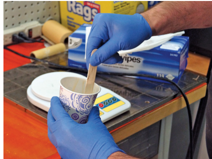
Figure B-3: Mixing the epoxy.
