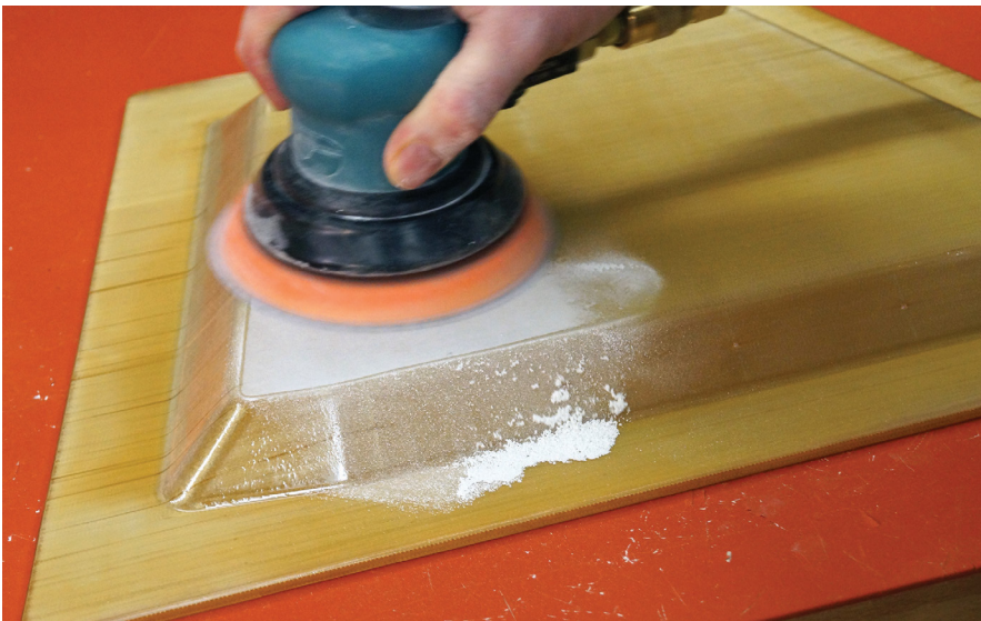
Figure B-1: Initial sanding of tool with 120-grit sand paper.
