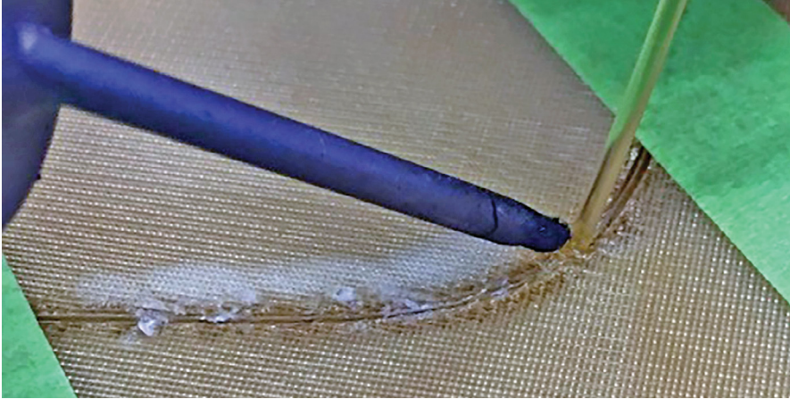
Figure A-5: Filament welding two sections together.
