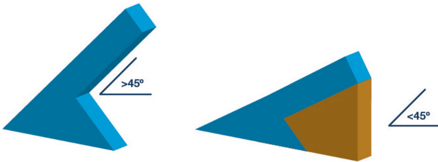
Figure C-5: Self-supporting angles (left) require no support material.
