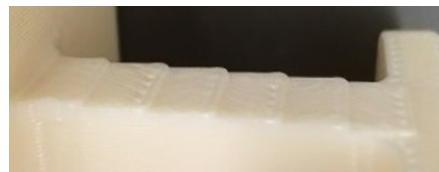
Figure C-8: Stair-stepping with a small slice height.
