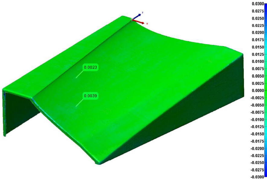
Figure 5-4: 3D scan data for a UAV fan-blade tool (shell style) after thermal cycling with color map comparison to the 3D scan data for the same tool prior to cycling. Dimensions are in inches.
