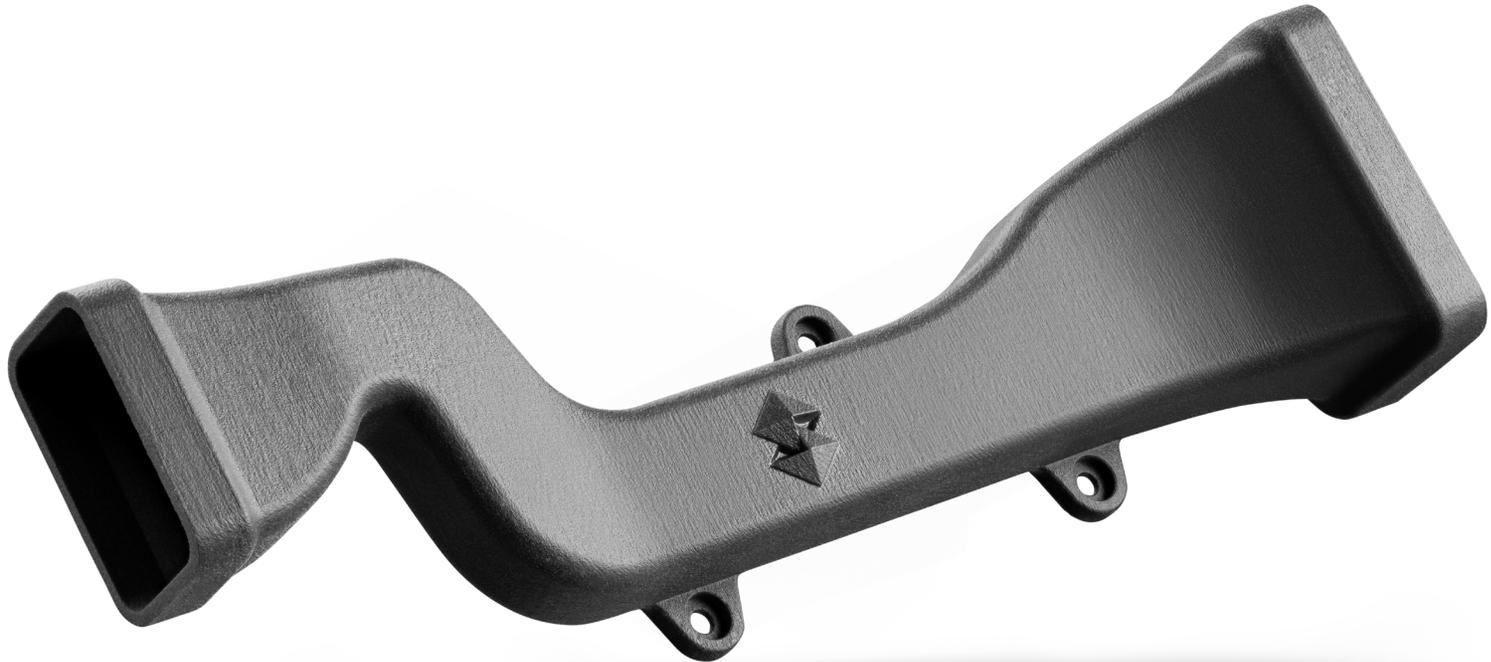
This air duct part of an automotive HVAC system, printed with SAF™ technology. Traditionally, a part like this might be molded as two halves and assembled. With SAF technology, the halves can be produced as a single part, reducing post process assembly and points of failure.
