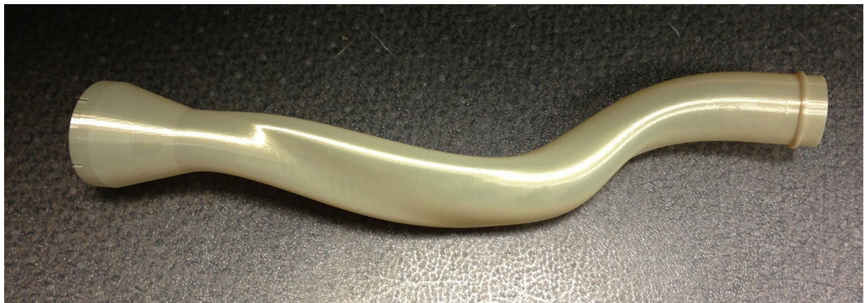
Figure 1: Ducts, in limited production runs and customized shapes, can be produced at a lower cost compared to traditional manufacturing methods.
