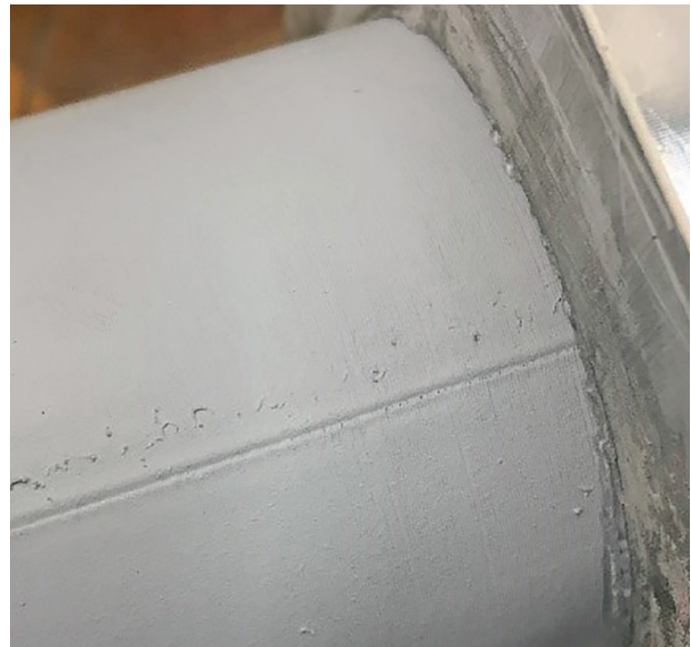
Figure 27: Standard aerospace or automotive paints formulated for plastics can be used to seal FDM ducting for low-pressure applications.
