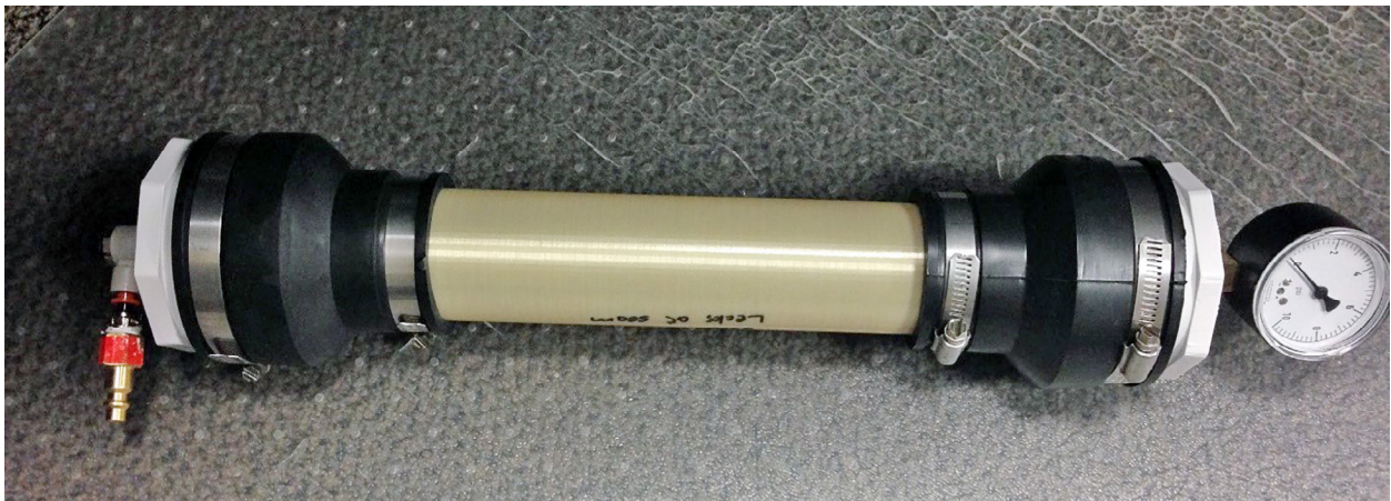
Figure 24: FDM parts exhibit a process-induced porosity that is undesirable in ECS ducting. If the pressure loss incurred from the presence of the porosity is not tolerable, use a secondary process to seal the parts.
