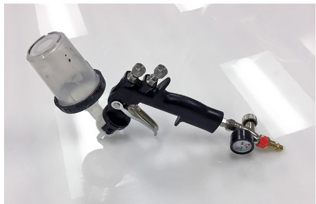
Figure 25: Spraying epoxy reduces the manual labor for post-process sealing compared to brushing.
