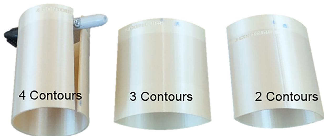
Figure 43: Post-test results when loaded to 1000 lbs (4448 N).
