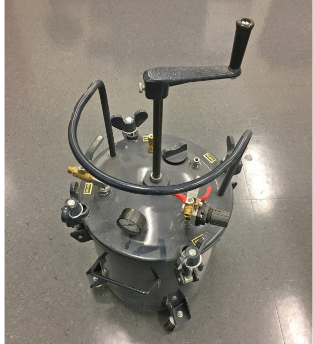
Figure 26: Vacuum impregnation can be performed using small vacuum pots or large industrial impregnation centers.
