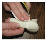
Figure 1: Hand sanding is one option for part finishing, but it may be prohibitive due to cost and time.
