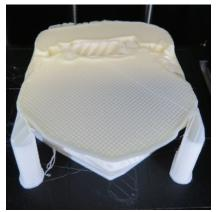
This partially 3D printed creature demonstrates the recommended sparse fill pattern.
