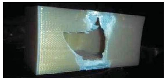
Figure 12 Real life test showed a part failure at 17 kg loading. The location of the stress concentration was the same as in simulation.
