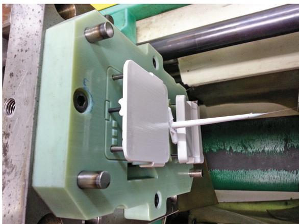
Injection-molded parts being ejected from a 3D printed mold.
