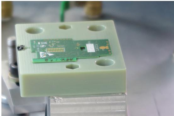
An example of a PolyJet low-pressure injection mold.
