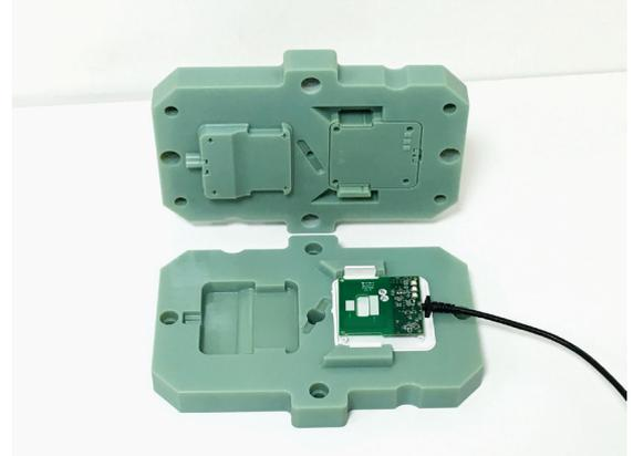
A 3D printed mold created in Digital ABS material by Arad Group.
