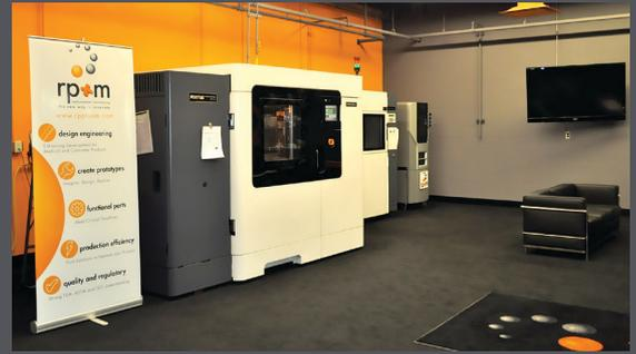
Three of rp+m's FDM additive manufacturing machines.
