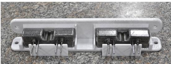
Even simple CMM fixtures can save hours in the inspection process.
