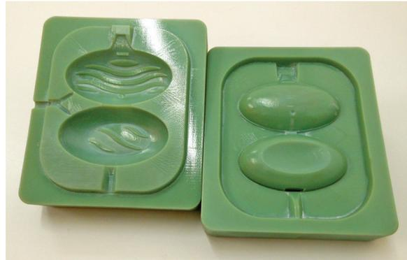
A 3D printed injection mold for a Domestos-brand toilet rim block
