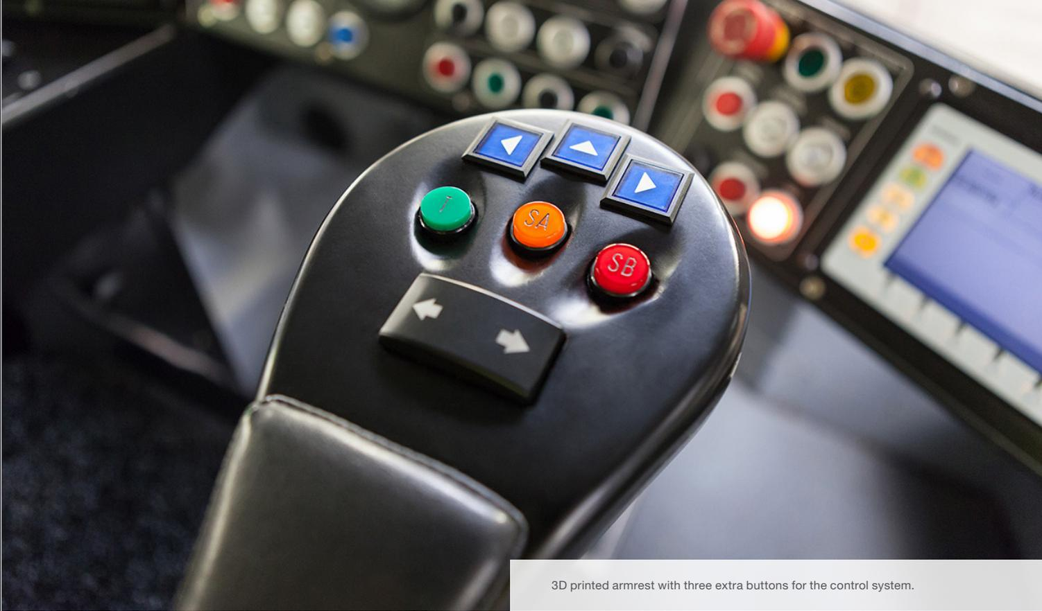
3D printed armrest with three extra buttons for the control system.
