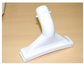
3D printed vacuum nozzle for the removal of any contaminating particles, produced using the Fortus 450mc 3D Printer.
