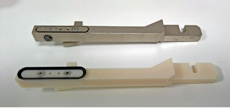
UPSA is making 95% cost-savings on just one part alone by replacing cast steel arms with high-performance 3D printed arms using ABS-M30i 3D printing material.
