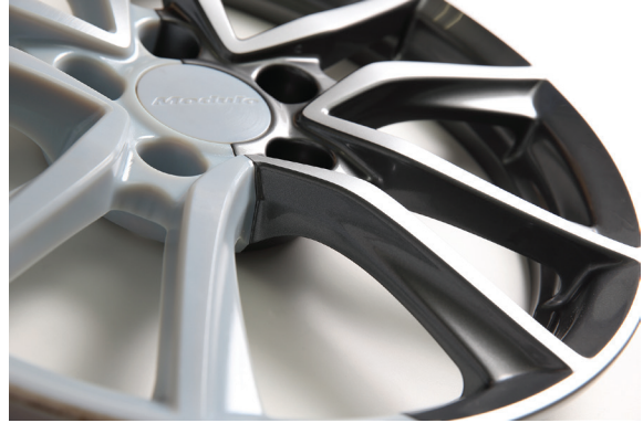
Wheel prototype model printed by Objet Eden500V: divided into few pieces and assembled.
