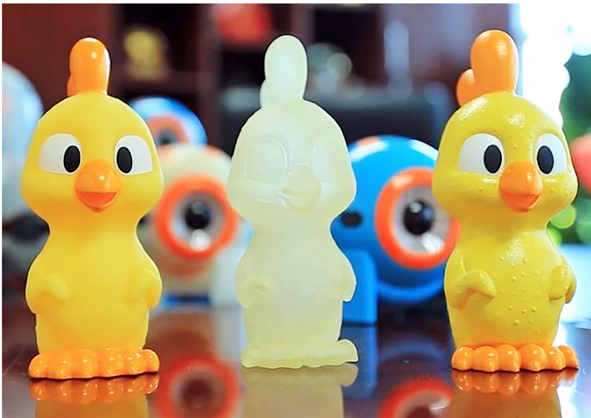
3D printed models (middle and right) shown with the final mass-produced product (left).
