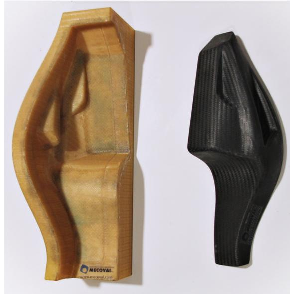
3D printed composite layup tool produced in ULTEM™ 9085 resin, alongside the final carbon-fiber part for use in Formula One racing.
