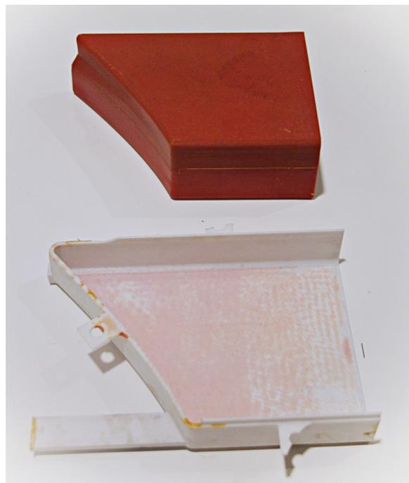
3D printed mold produced using Stratasys polycarbonate material, used to produce the polyurethane part in red for the automotive industry.
