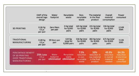
Fig. 1 - Comparison of outputs from the traditional and 3D printing approaches
