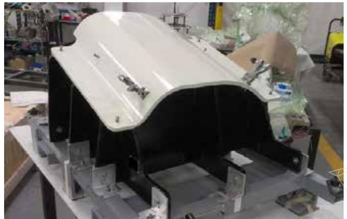
Figure 11. FRP machining fixture for the speaker box panel.
