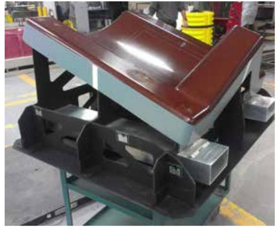
Figure 8. Speaker box FRP mold.
