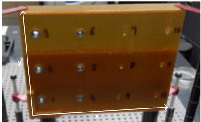
Figure 4. View of the printed geometry with inserted bushings. Solid arrows indicate measurement direction.
