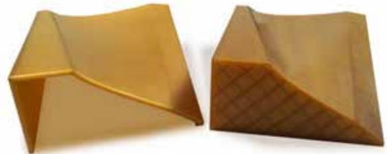
Figure 2. FDM tool construction styles.
