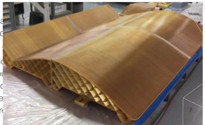
Figure 15. Assembled 4-piece FDM cabinet headliner lay-up mold.
