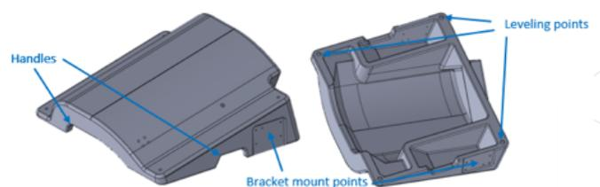
Figure 12. Views of the FDM speaker box machining fixture design.
