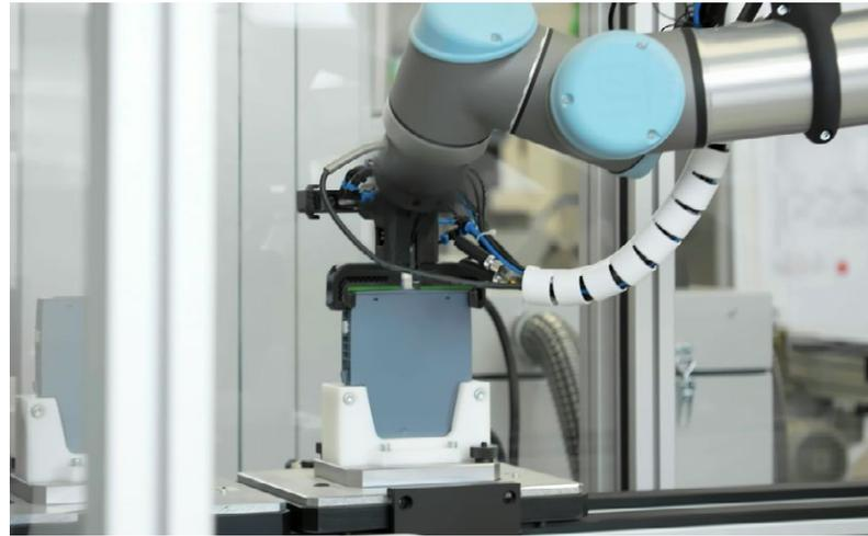
For the robot grippers, additive manufacturing enables the compact design, and applications such as complex vacuum channels in the basic body can be realized.
