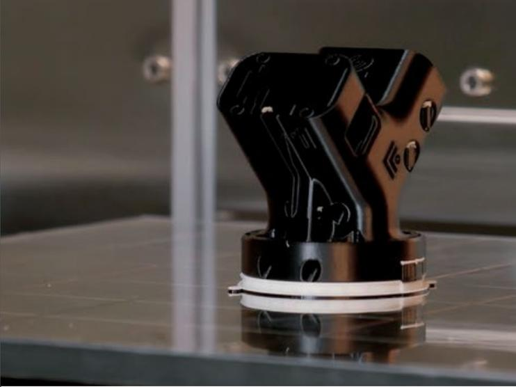
Stratasys offers additive manufacturing materials that comply with European ESD standards and enable reliable and repeatable 3D printing, such as this robot gripper.
