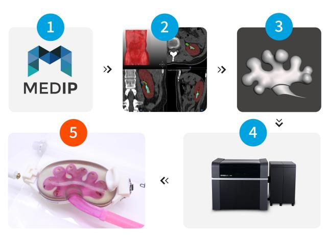
The process of printing a 3D model of kidney images, with segmentation performed by the MEDIP software of MEDICAL IP to create a 3D training model for retrograde intrarenal surgery (RIRS) using the Stratasys J750.
