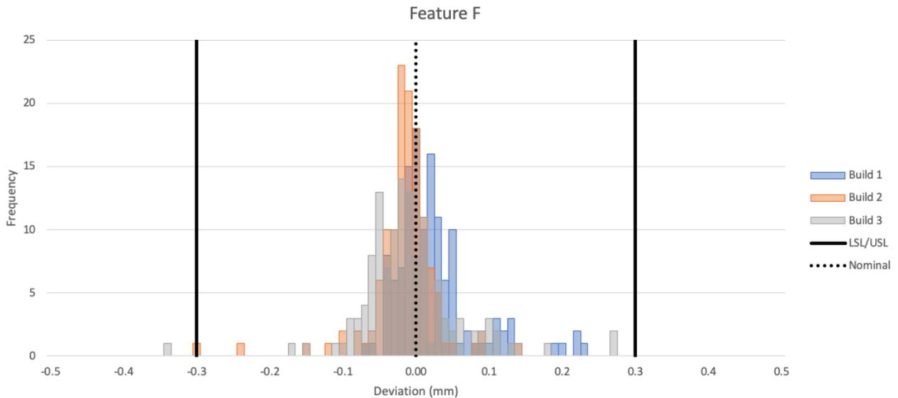
Feature F shows a broad spread, with a few outlier specimens in the extremes of the histogram. The peaks lie within 40 $\mu$ m of each other. It achieves an overall yield of 99.7%, a CPK of 1.6 and the spread is consistent with IT14.
