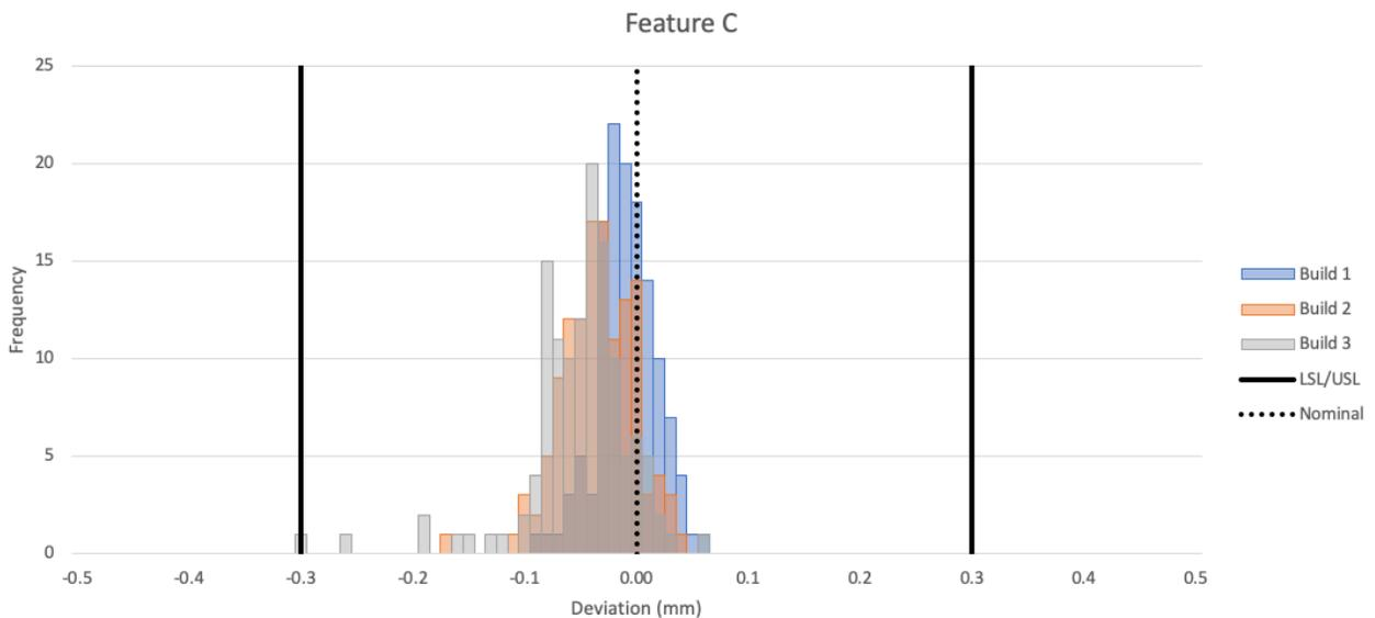
Feature C is very well centred and features minimal outliers. The range between histogram peaks is  $42\mu\text{m}$  and the feature overall achieves a yield of 100%, a CPK of 2.2. The spread is consistent with IT13.
