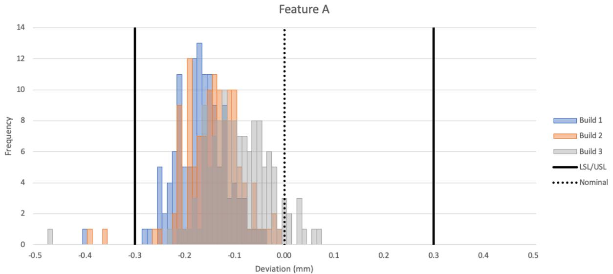
Feature A is mostly in spec but contains some outliers below the lower spec limit (LSL). The individual builds are consistent, with the mean deviation (peak of the histogram) from each build within 75 $\mu$ m. Overall, the feature achieves a 99.0% yield with a CPK of 0.9 and the spread remains consistent with IT15 according to ISO286-1.
