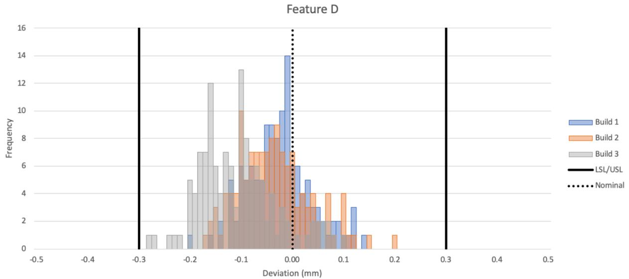
Feature D exhibits a much broader spread than the previous features but is still consistent within builds. It has a range of histogram peaks of  $81\mu\text{m}$ . It also still achieves an overall yield of 100%, a CPK of 1.1 and the spread is consistent with IT15.
