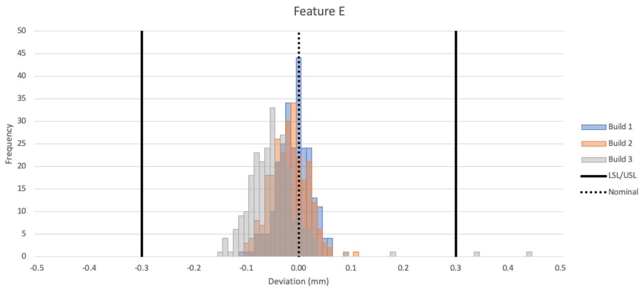
Feature E shows upwards outliers, some of which lie outside the upper spec limit (USL). The consistency between builds is still good, with the range of histogram peaks lying within  $39\mu\text{m}$  of each other. It achieves an overall yield of 99.7%, a CPK of 2.1 and the spread is consistent with IT14.
