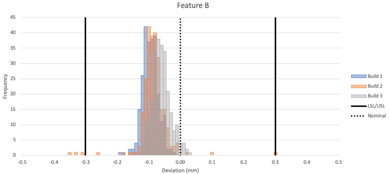
Feature B signifies many of the same behaviors as feature A. This shows tight grouping between builds and a few low outliers that lie outside of the LSL. The histogram peaks all lie within  $35\mu\text{m}$  of each other and the feature overall achieves a yield of 99.5%, a CPK of 2.0 and the spread is consistent with IT14.
