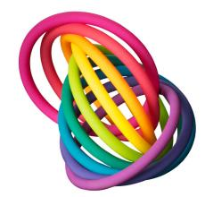
Figure 9: These interlocking color rings were 3D printed in one job using the cyan-magenta-yellow palette.
