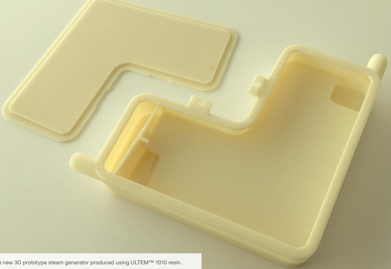
Part of the new 3D prototype steam generator produced using ULTEM™ 1010 resin.
