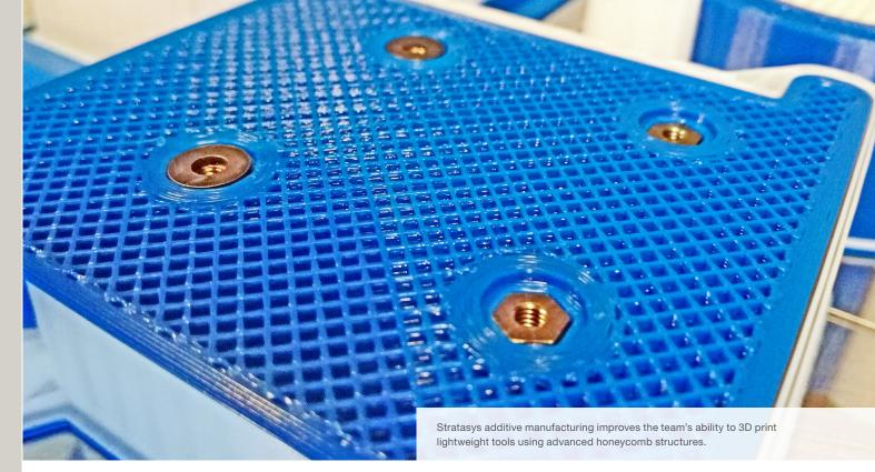
The company purchased a Stratasys® FDM® 3D printer to seamlessly and cost-effectively respond to industrial needs with advanced tooling. Requiring an easy-to-operate, safety-compliant solution that would keep up with production demands, Hager chose the industrial-level Fortus 380mc™ 3D printer. This high-performance 3D printer enabled the company to work with production-grade thermoplastics.
