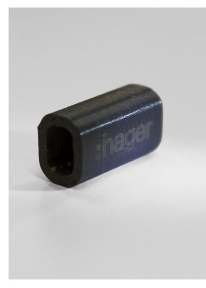
Final 3D-printed cap for use with an electronic device produced in ABS-M30  $^{\text{TM}}$ .
