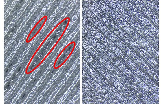
Magnified images of ABS-CF10 with porosity (bead gaps) circled on the left and no gaps after tuning with OpenAM on the right.
