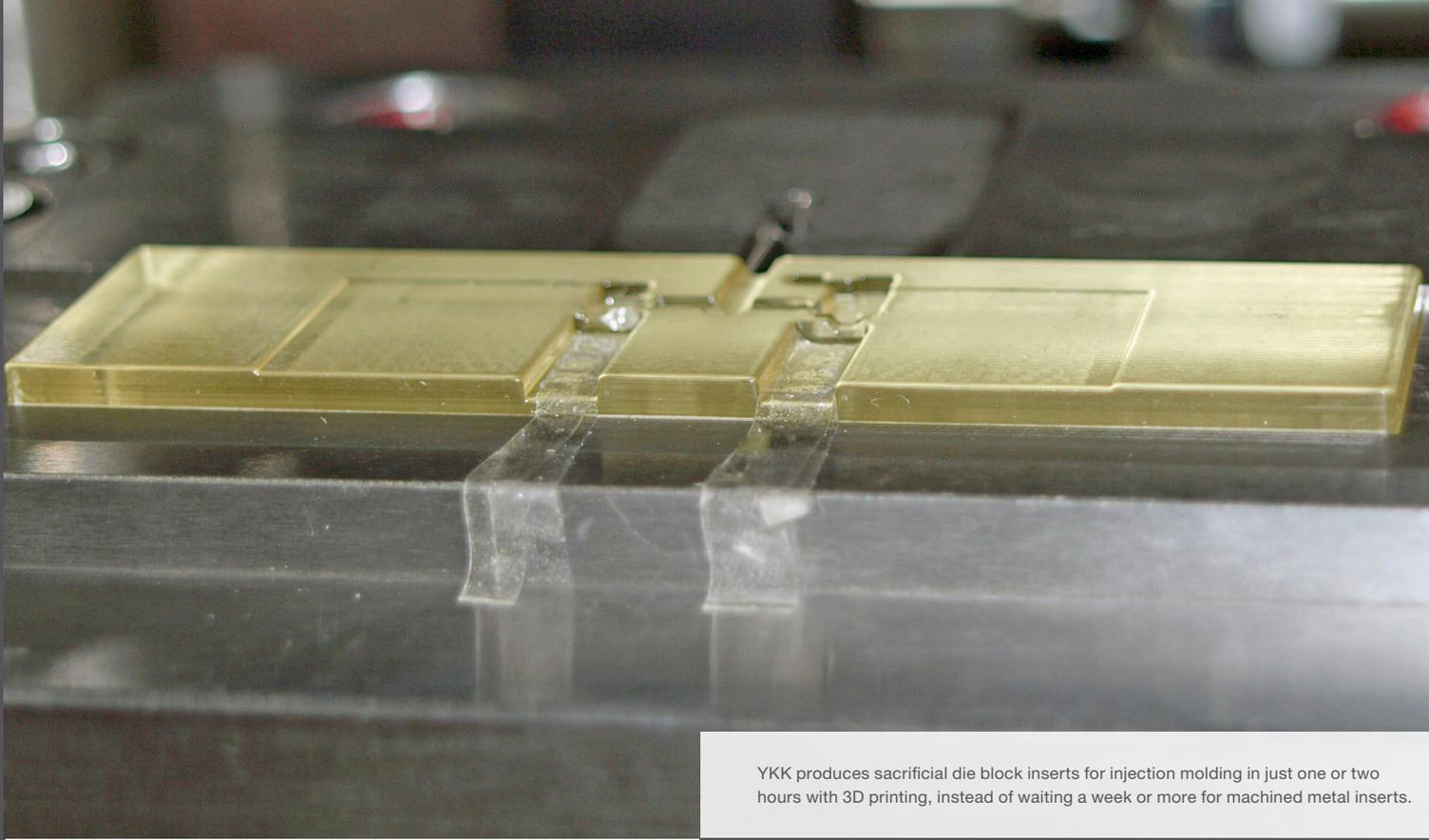
YKK produces sacrificial die block inserts for injection molding in just one or two hours with 3D printing, instead of waiting a week or more for machined metal inserts.
