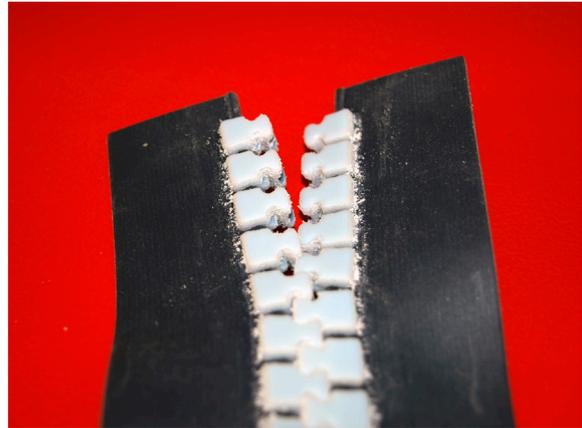
This oversized example of zipper teeth was 3D printed on the Connex3 to demonstrate the function of a new design concept.
