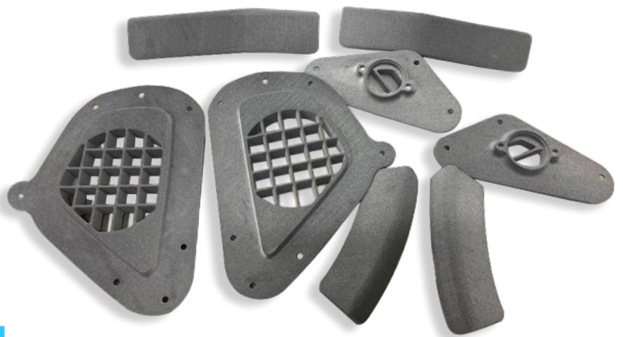
Interior parts printed using SAF technology.
