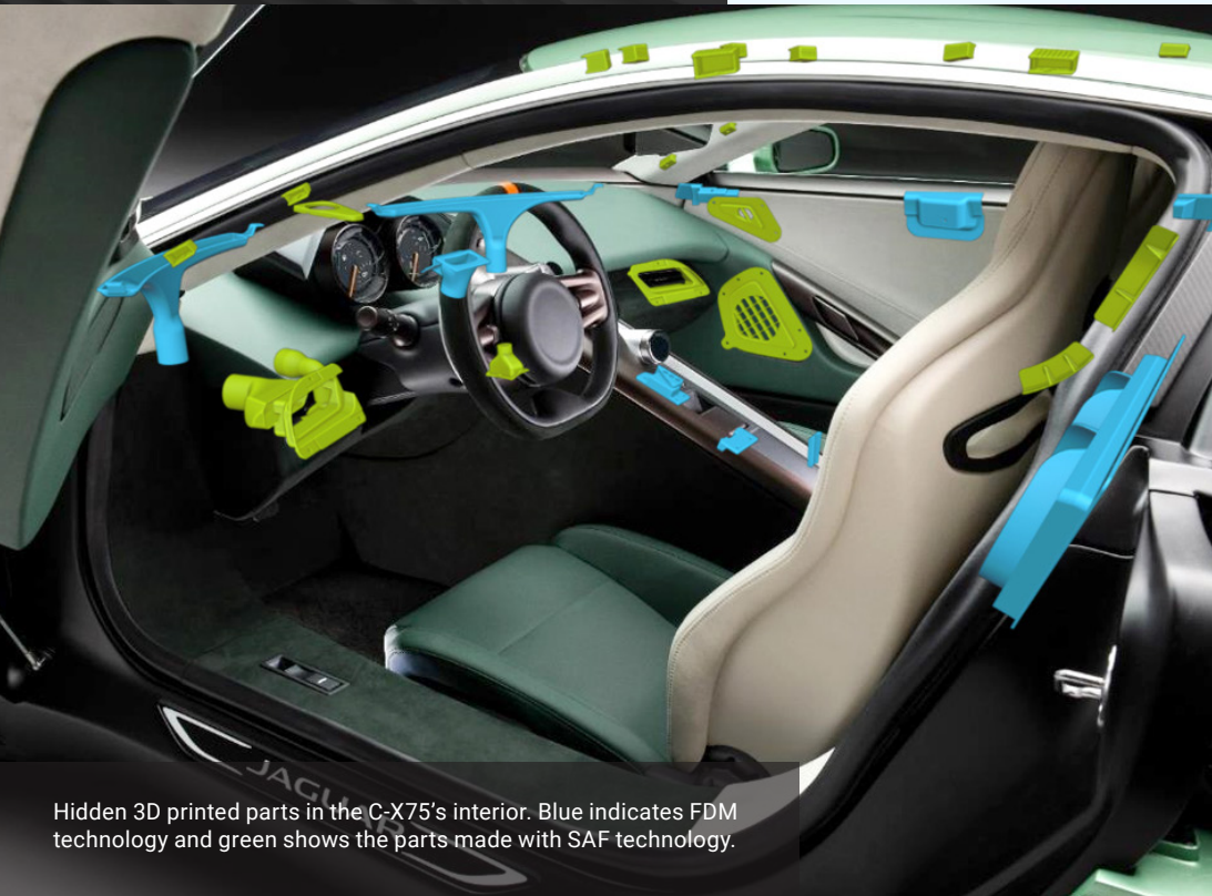
This schematic shows the 3D printed parts used in the interior. FDM technology parts are blue, SAF technology parts are green.
