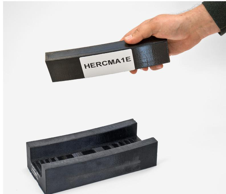
3D printed forming tool in Stratasys Nylon 12.
