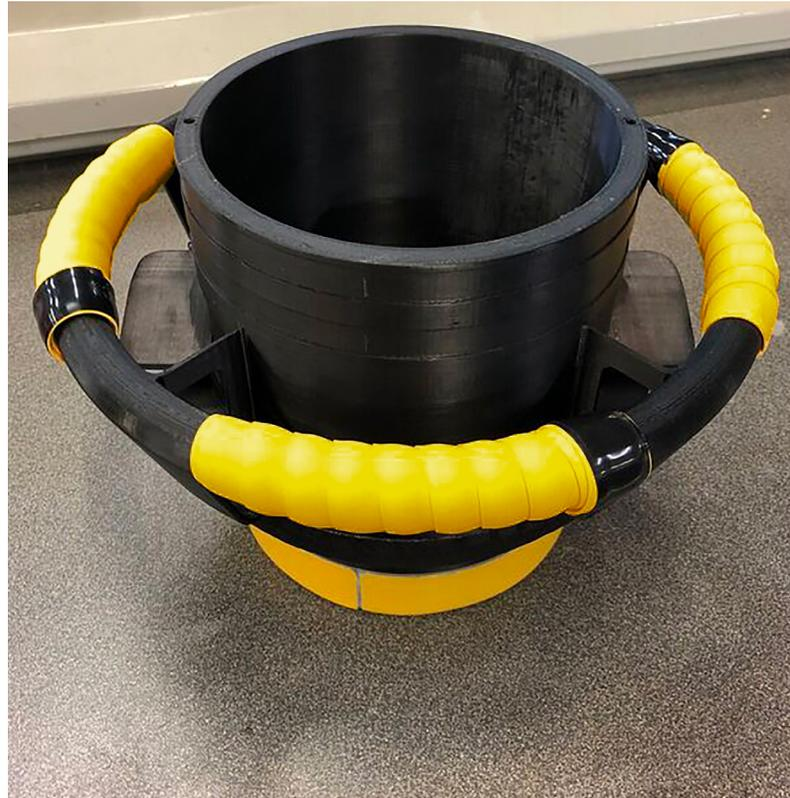
Final, 3D printed ECS duct adapter designed to cool aircraft while on the ground. 3D printed in Stratasys FDM Nylon 12 on the Fortus 450mc.
