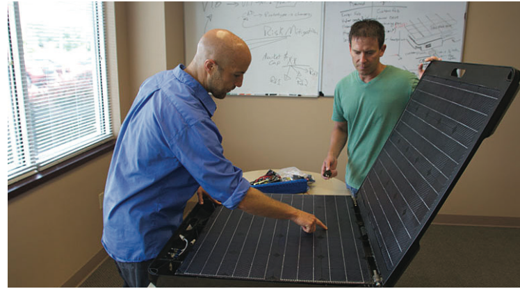
A 3D printed prototype made of strong ABS plastic helped Peppermint Energy design its FORTY2 solar generator .
