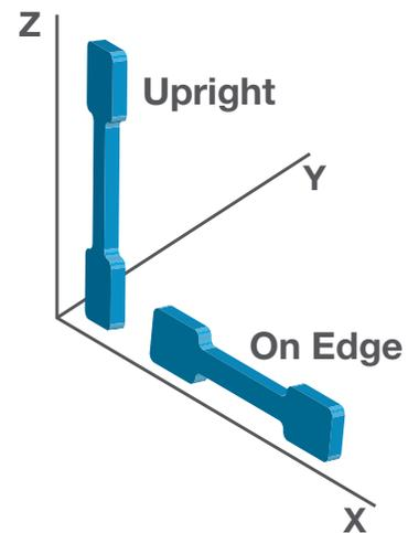
Figure 1: Test sample orientations
